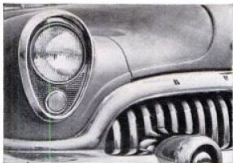
BUICK has moved its parking lights from inside the bumpers to a safer position beneath the headlights
