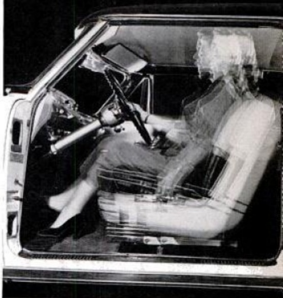
LINCOLN front seats move up and down as well as forward and backward. Electric motors do the work!
