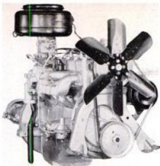
PLYMOUTH uses a six-bladed fan this year. Diameter is smaller and fan speed decreased. Change was made necessary by lower hood line
