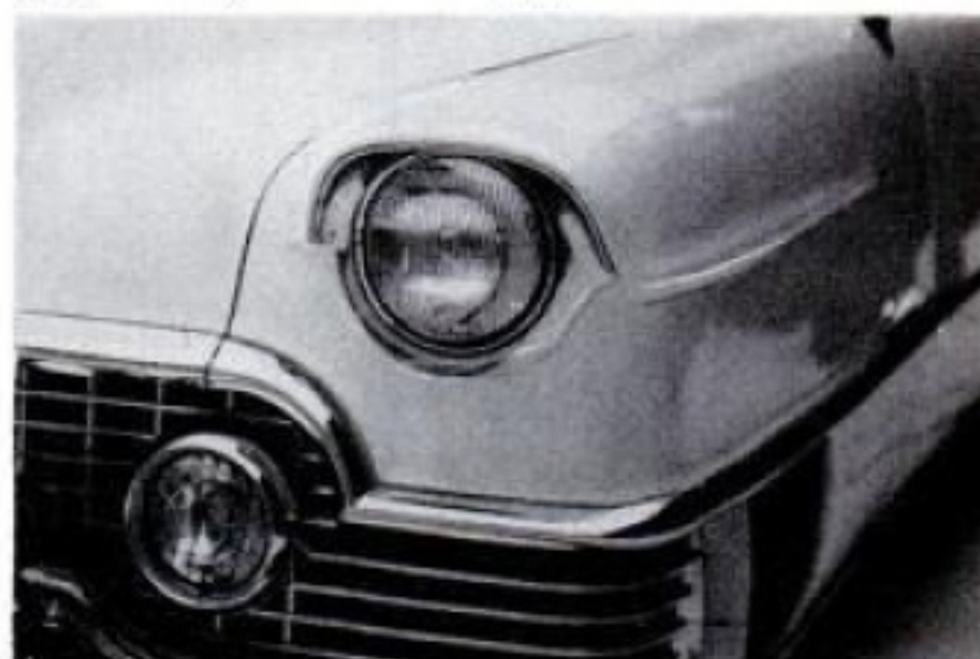
CADILLAC has enlarged the "eyelid" over its headlight, forming it with the top part of the fender
