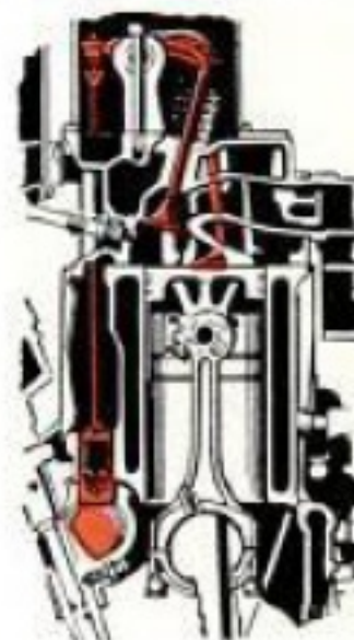
CHEVROLET's new 125-hp. engine has high-lift cams
