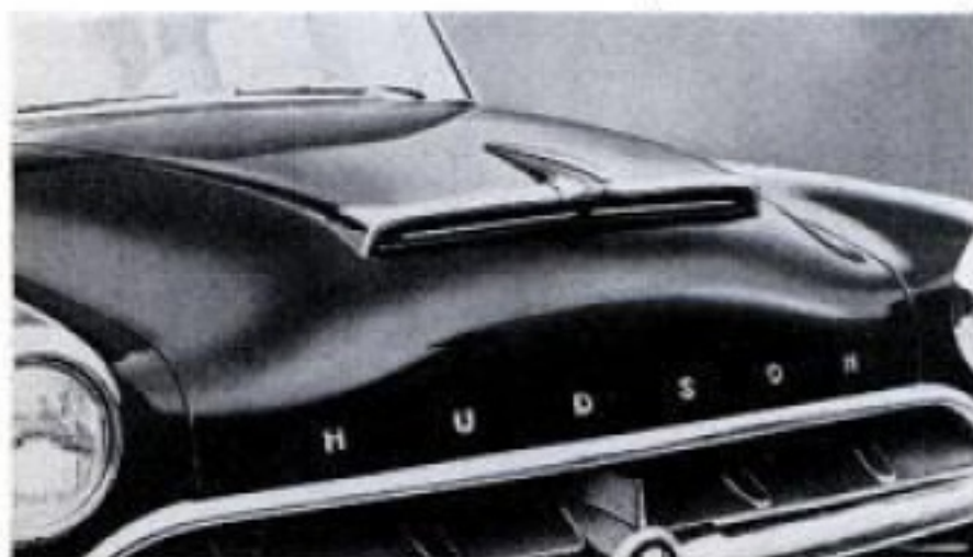
HUDSON lowered its hood and added a broad air scoop that admits air into top of engine compartment
