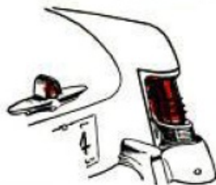
MERCURY extended its rear fenders over the top of the taillight unit
