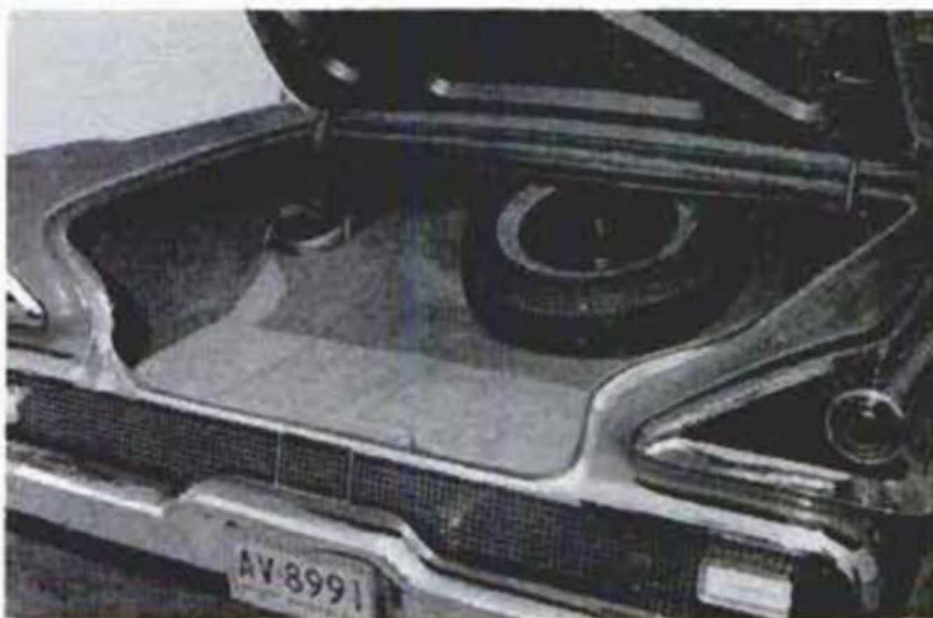
Spare mounts forward to increase handy-to-get-at trunk area. After all, when did you last need a spare? Below, frame cross-member over rear axle is curved heavy-gauge sheet metal instead of box girder. It is lighter, stronger, requires less height
