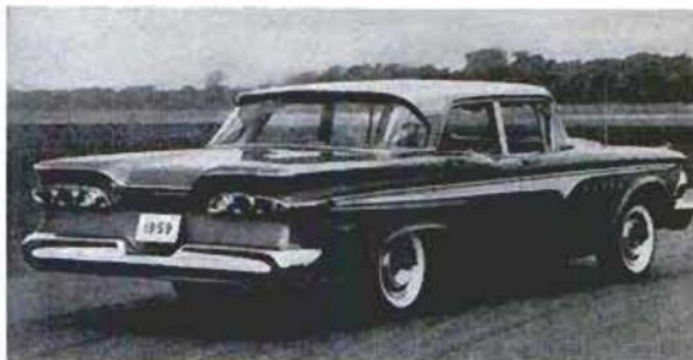
Ranger sedan is same size inside and out, but less expensive than Corsair. Differences are in trim, seat design and engine
