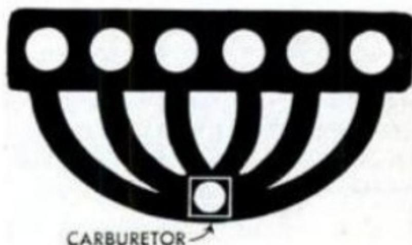
Usually, an inline six manifold is the "log" type, upper drawing, with sharp corners. Valiant's is a "bunch of bananas" with gentle curves, lower drawing, that give excellent breathing to all six cylinders
