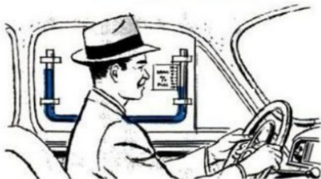
Performance meter is made by taping a transparent plastic tube to window and adding colored water
