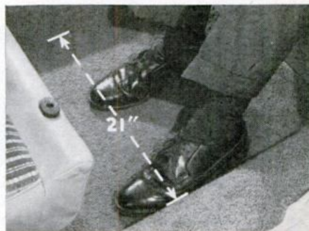
FORD GALAXIE'S new perimeter frame provides wider cabin well for more foot room, especially in front. Top photo rear in '64, lower one a new '65
