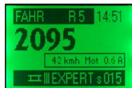
Typical RailCom messages during the initial phase in the LOCO-OPERATOR mode
